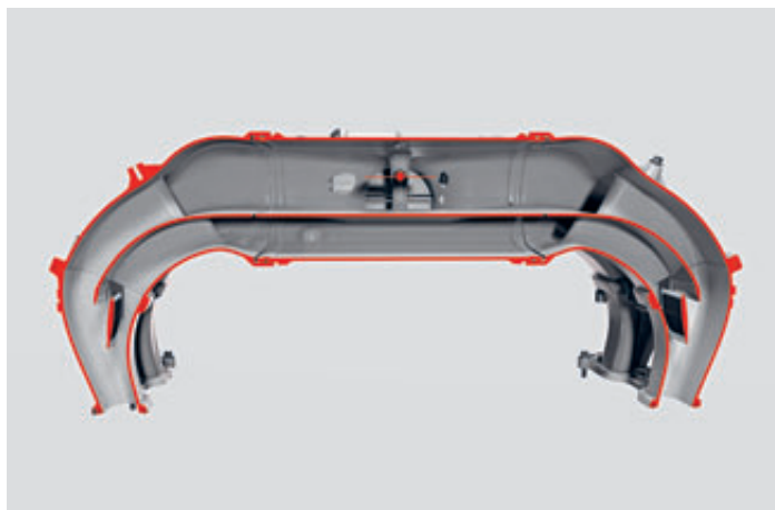
Improved torque curve in partial load operation: The cast aluminum intake system has a tuning flap in the receiver volume that enables separation of the two cylinder banks.
