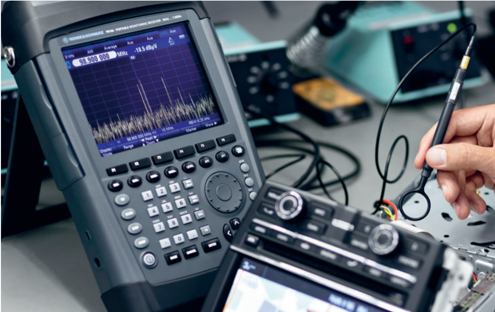
Analyzing the interference sources and testing the switching paths for a vehicle component
