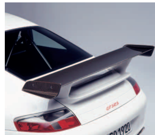
The large rear wing provides the 911 GT3 RS with increased downforce at the rear axle.
