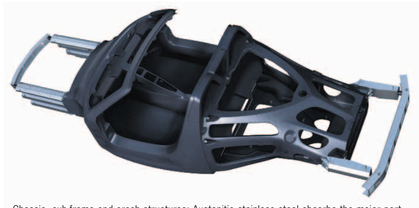
Chassis, sub-frame and crash structures: Austenitic stainless steel absorbs the major part of the energy acting on the vehicle in a crash.
