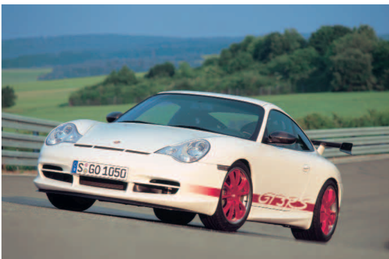
Special openings in the front section deliberately direct the exhaust air from the radiators over the vehicle.
