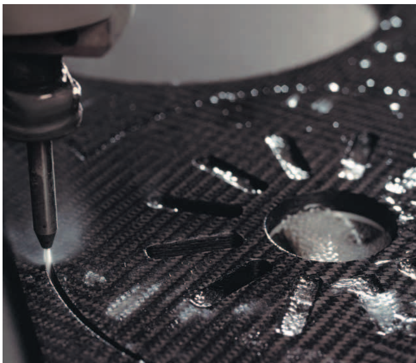
A water jet cuts the friction disk out of the ceramic plate at around 3,000 bar.
