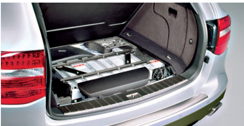
Cayenne hybrid with nickel-metal hybrid battery (NiMH)
