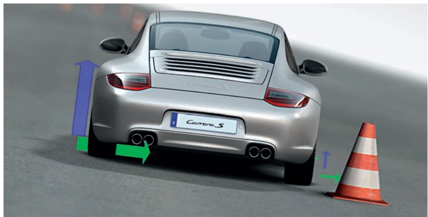
The virtual car in motion. Properties such as wheel forces which are not directly visible are indicated by arrows
