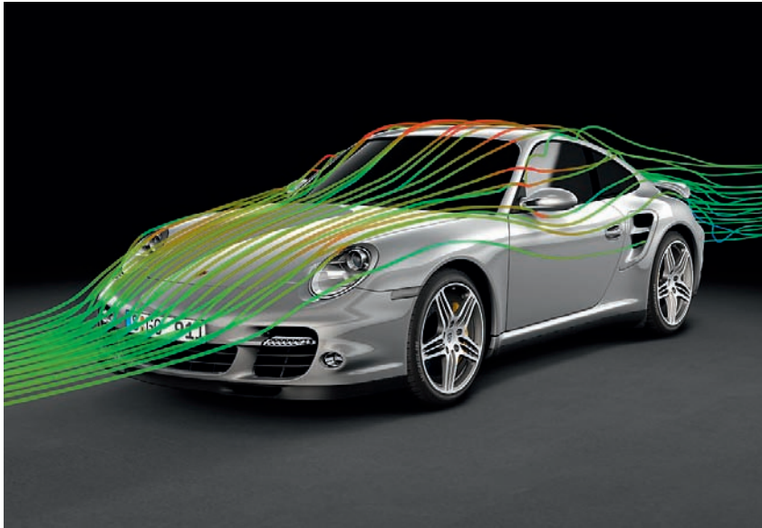
Realistic visualization of flow simulation data: Physical processes such as air flow distribution are made visible on the design model
