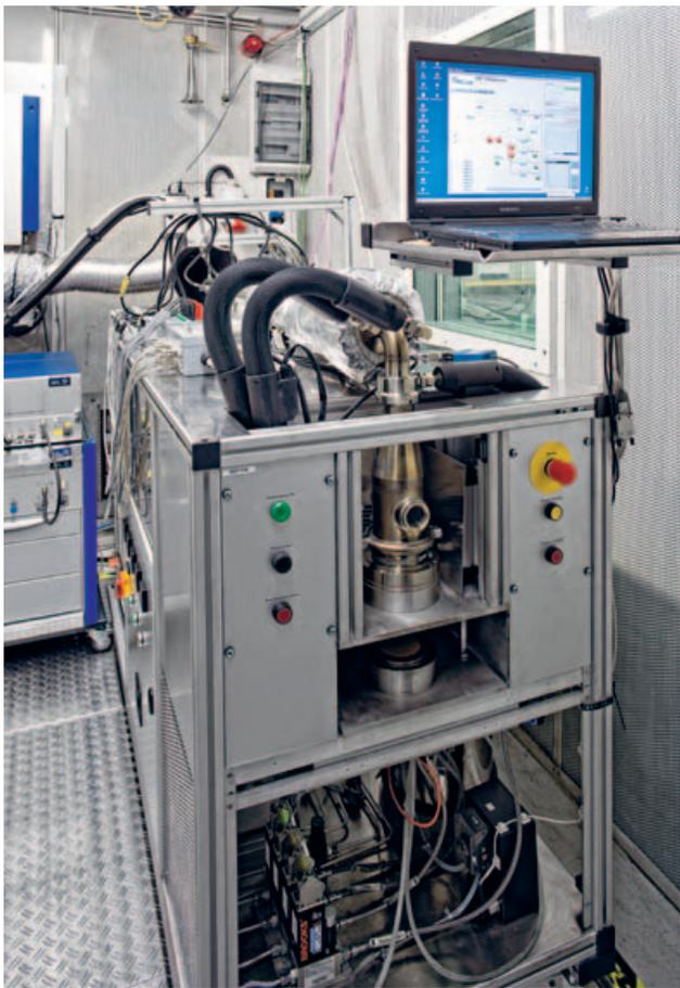
ADA test bench for testing exhaust emissions
