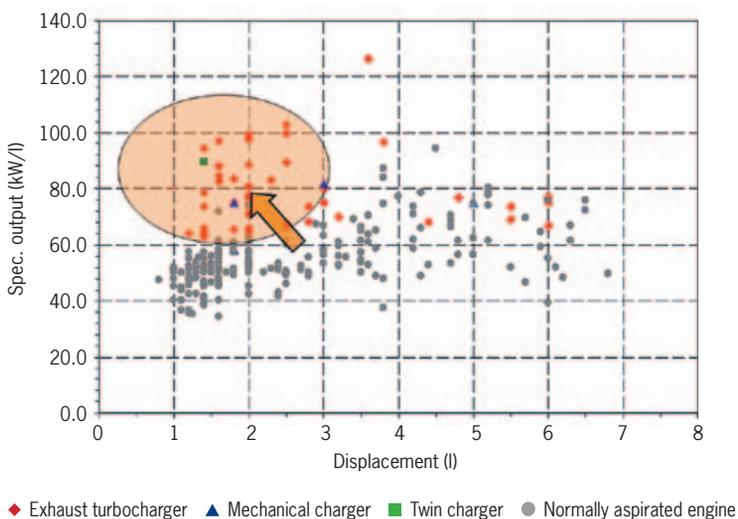
*Due to engine downsizing, high specific output is possible with reduced displacement.*
