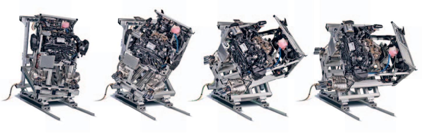
*The tilt test bench enables biaxial rotation of up to 60 degrees in any direction.*
