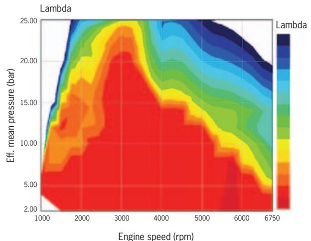
Lambda engine characteristic map of a 1.6-liter turbo engine with mechanical charger
