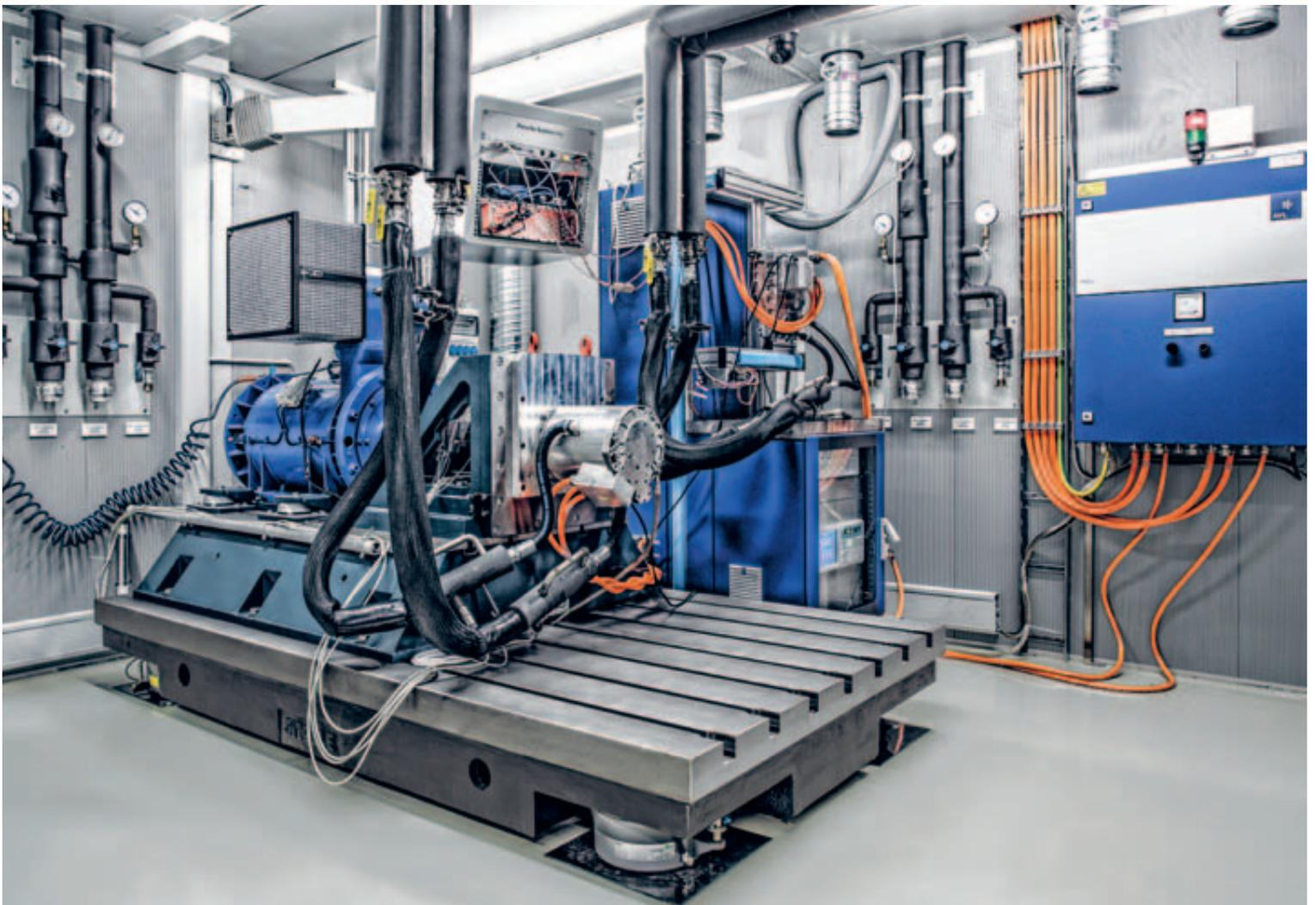
*When using the test bench, the electric motor can be operated either with a universal inverter or with the inverter that will later be used in the vehicle.*
