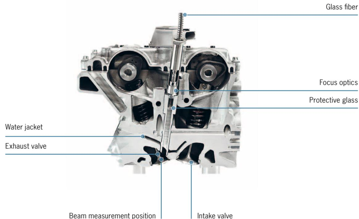
Sensor integration in cylinder head of a Porsche 911 engine
