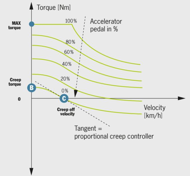
**Torque curves (vehicle velocity view)**
