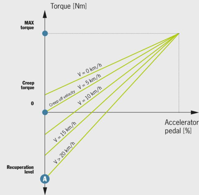
**Torque curves (accelerator pedal view)**
