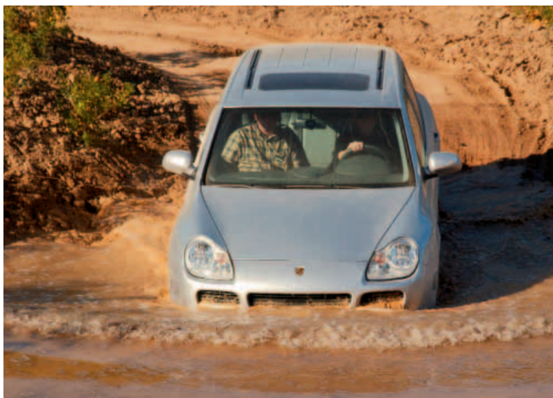
Bodies of water up to 555 millimeters deep are no problem for the Cayenne with air suspension.
