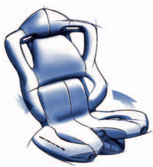
The initial design sketches are scanned and then edited in color with an electronic stylus.
