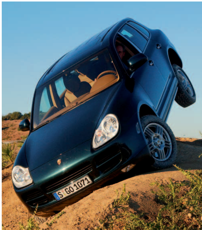
The high static torsional rigidity of 36,900 Nm/° gives occupants a feeling of safety and solidity, even when one wheel is hanging in the air.
