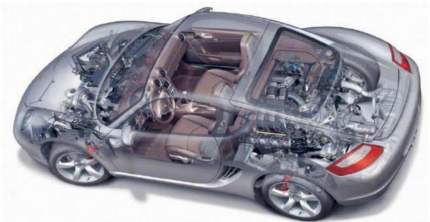
The mid-engine concept gives well-balanced weight distribution
