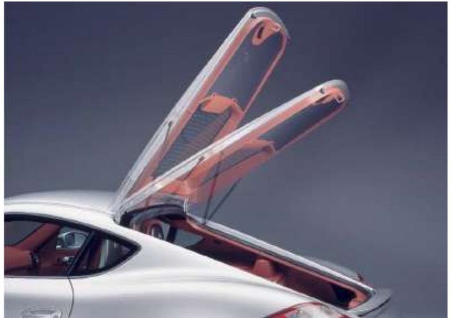
The large rear lid measuring 116 by 90 centimeters opens effortlessly with the aid of two stage gas springs
