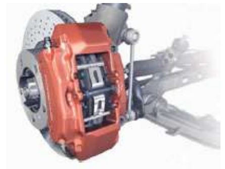
Brakes use four-piston monobloc calipers clamping internally ventilated disks
