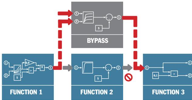
at the top of the page). A new function is coupled with the existing functions of the ECU. Internal values are made available to the bypass function as inputs. The output values are written to the memory cells of the variable or function to be replaced. In an external bypass, additional electric inputs or outputs can be fed into the function via special I/O hardware.
