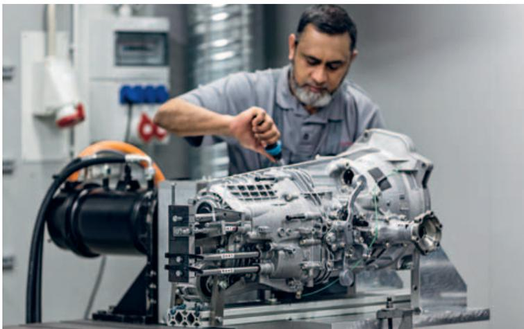
*A transmission is mounted on the test bench.*
