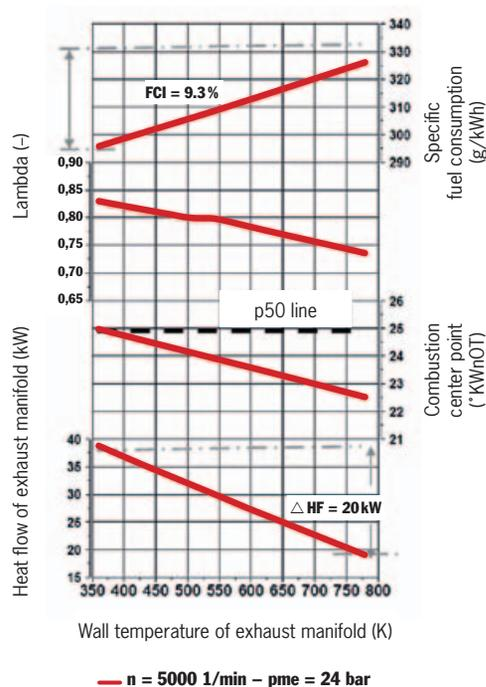
Fuel consumption improvements (FCI) through cooled exhaust gas recirculation
