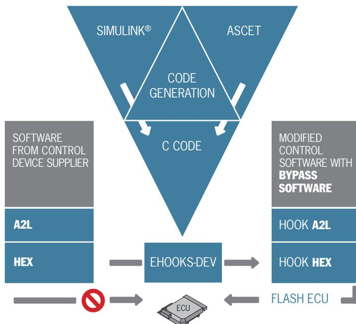
In the first step, just as with the internal method, the bypass hooks and the signals to be read must be set up with the EHOOKS-DEV application. This defines an interface to the future bypass software. The program code created with a build process with EHOOKS-DEV can be flashed onto the production ECU. This software solely contains a service for the ETL interface for exchanging data with the target. If the interface is to provide other data, the first step must be repeated.
