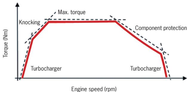
Limitations of single-step exhaust turbocharging
