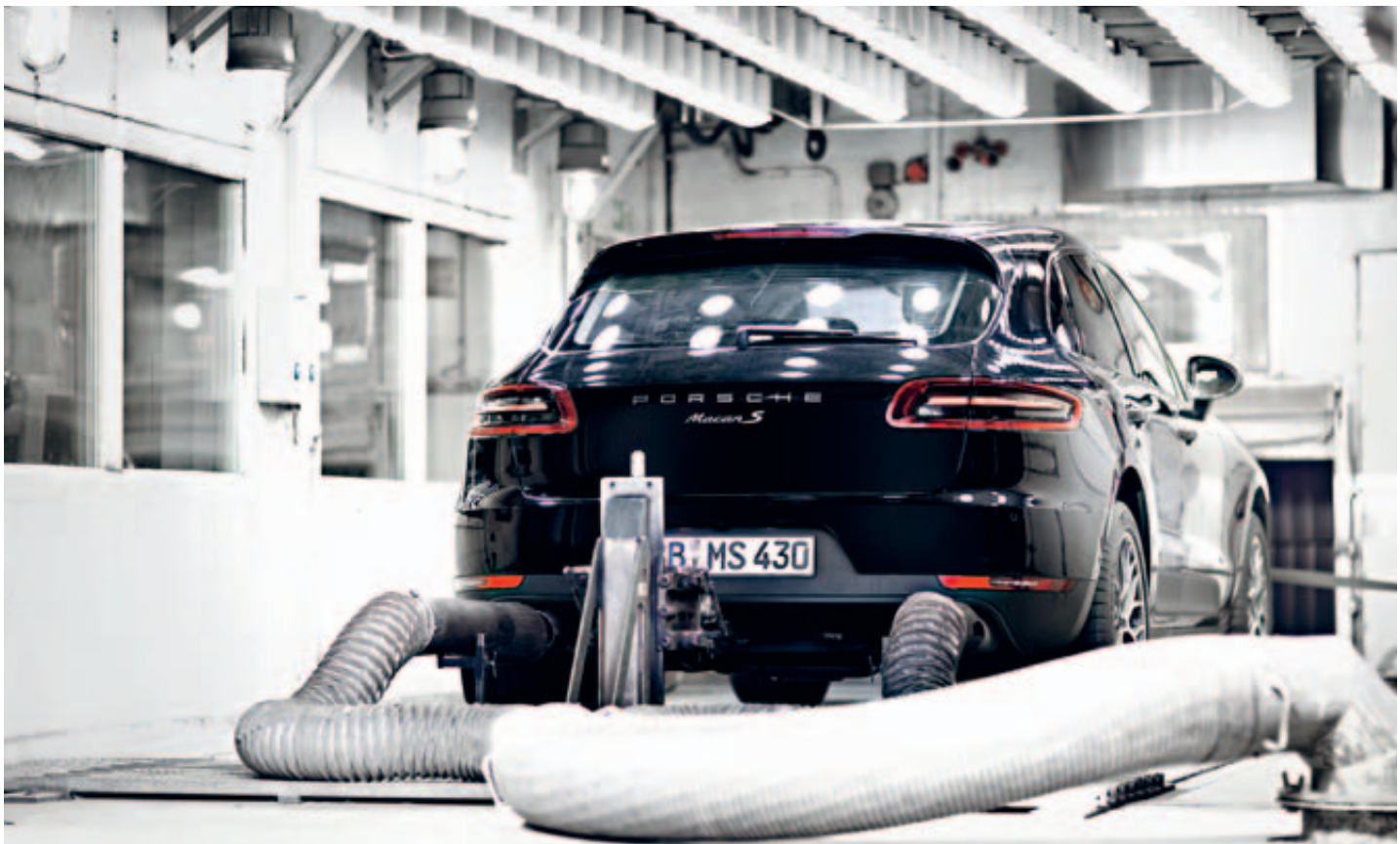
An essential part of the development of every vehicle: testing in a climatic wind tunnel
