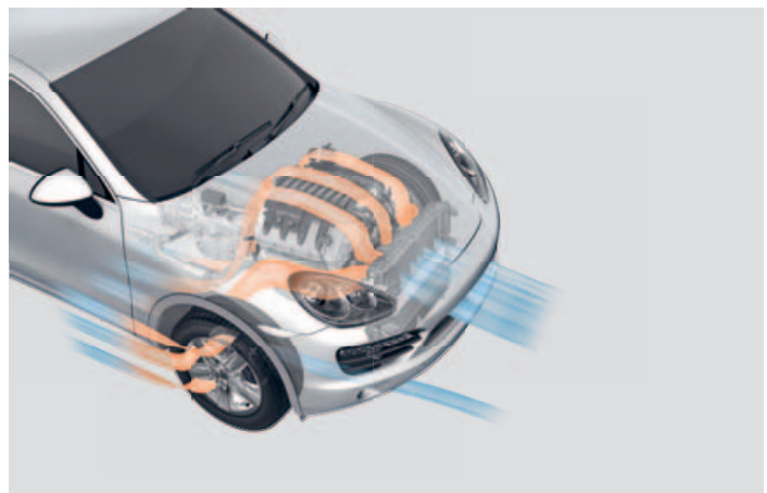
Efficient cooling air flow reduces the overall air resistance.
