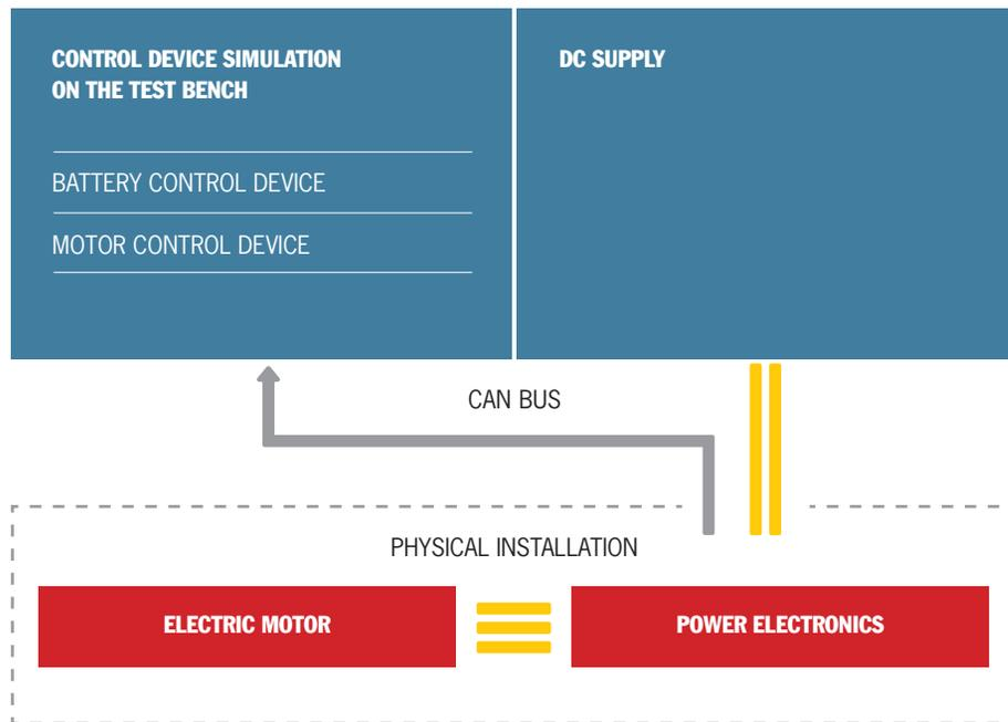
*Simulation of relevant CAN nodes from the vehicle on the test bench*
