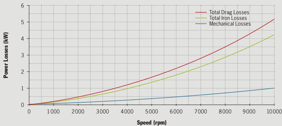
Figure 6: Drag losses across the rotary speed range
