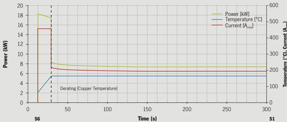
Figure 8: Development of power, current and temperature
