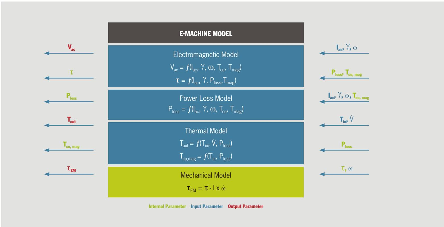
Figure 2: Building blocks of an electric machine model
