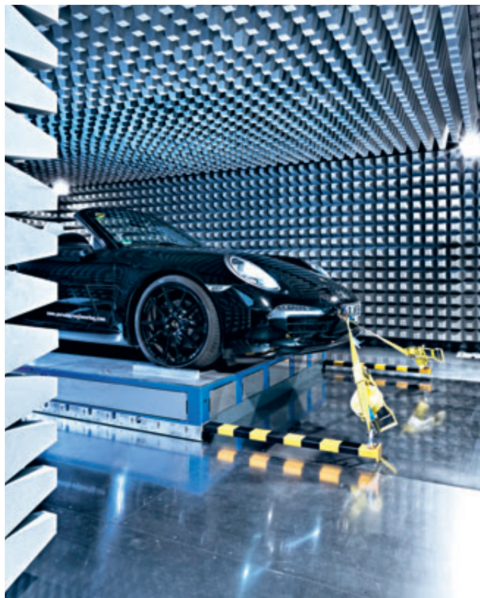
The new generation of the 911 Carrera Cabriolet is tested on the roller dynamometer
