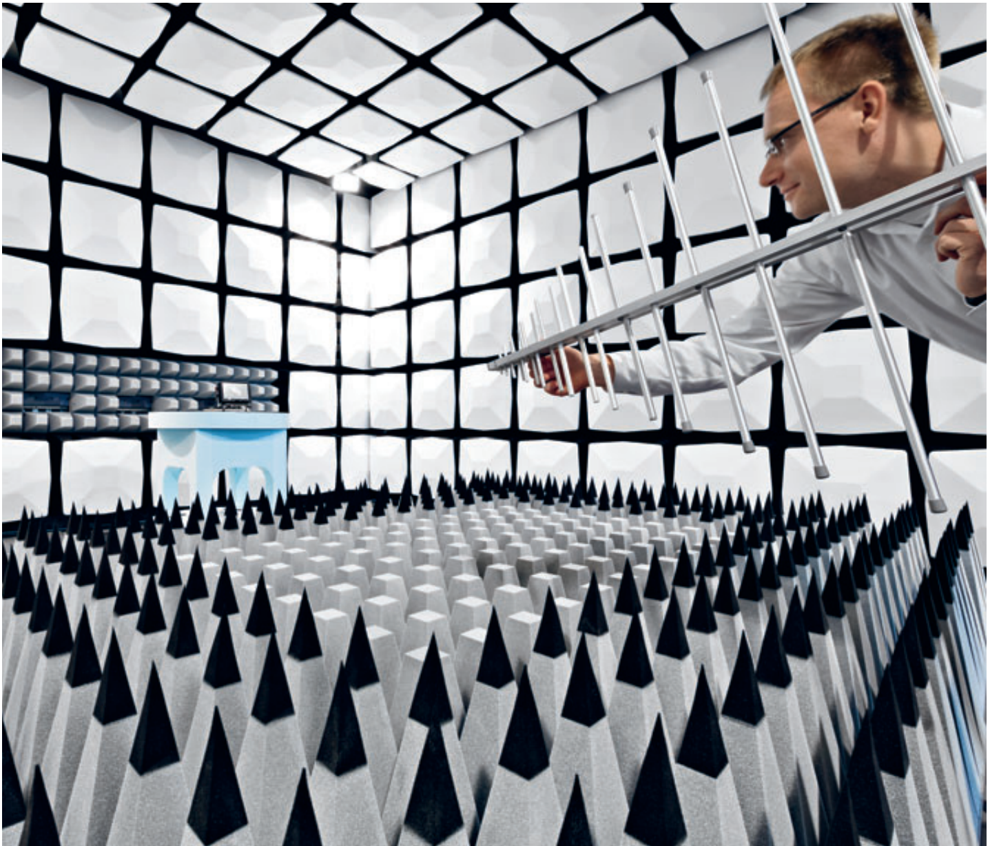
An interference emission measurement is performed in the anechoic chamber
