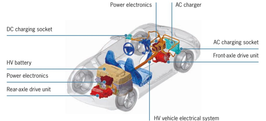
Overview of high-voltage components in the vehicle
