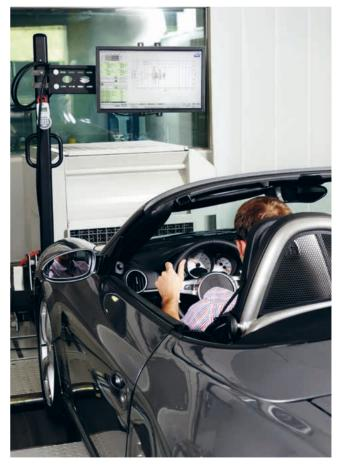
Measurement procedure on the roller test bench
