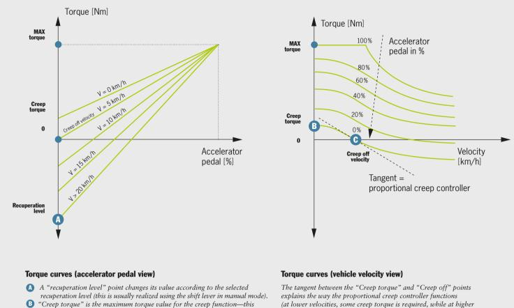
The conditions governing the application of torque are quite complex and the customer is largely free to define the dynamic vehicle response according to requirements. For example, the complete accelerator pedal/speed/torque curves can be changed. These curves have been simplified for their depiction in the figure on page 47.
