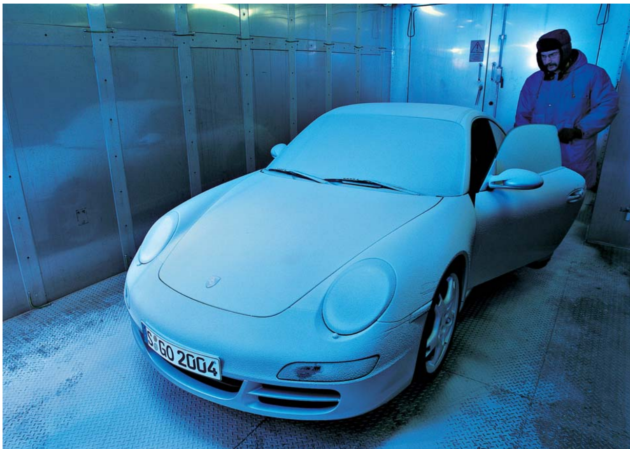
The 911 Carrera S under a sheet of ice: tests can be carried out at temperatures as low as minus 40 degrees celsius in the climatic chambers.
