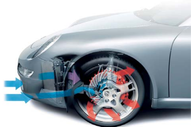
The cooling air channel at the front of the vehicle has been further optimized to reduce flow losses.
