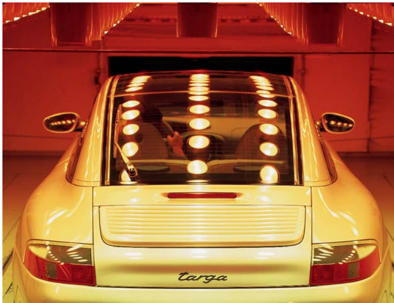
In the climatic wind tunnel, solar simulation can also provide sun-load to the Targa interior.
