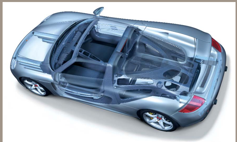
Both the monocoque as well as the entire sub-frame are constructed from carbon fiber reinforced plastic (CFRP).
