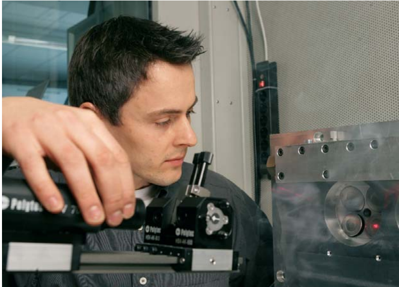
In order to take measurements, the laser beam is positioned to meet the valve head vertically.
