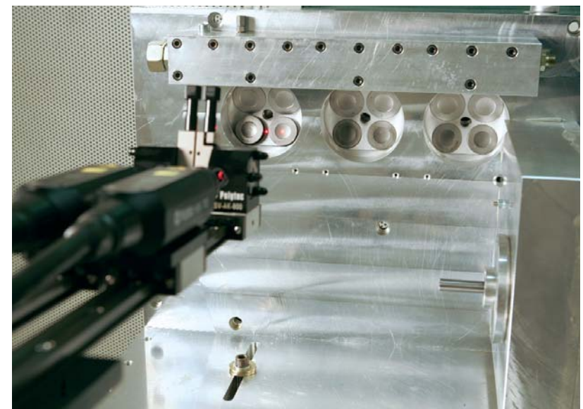
A second laser beam is positioned as a reference measurement beam parallel to the first and adjacent to the valve seat to measure the relative movement of the valve.
