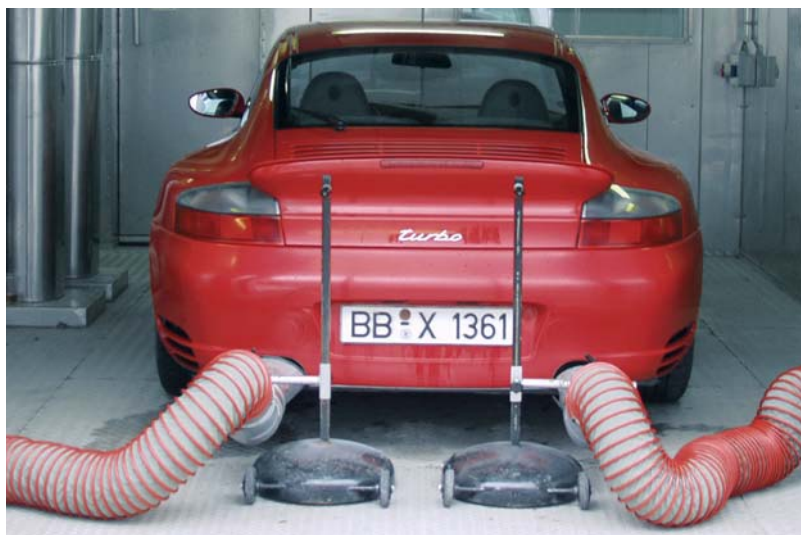
During driving simulations or as in this case cold start tests a special system draws off the exhaust gases.
