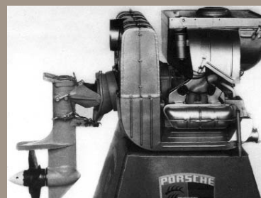
The engine of the Porsche 356 was modified for the use in water.
