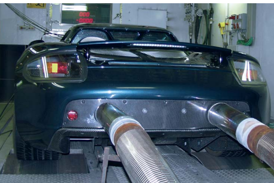
Testing the air conditioning of a prototype of the Carrera GT in the climatic wind tunnel.
