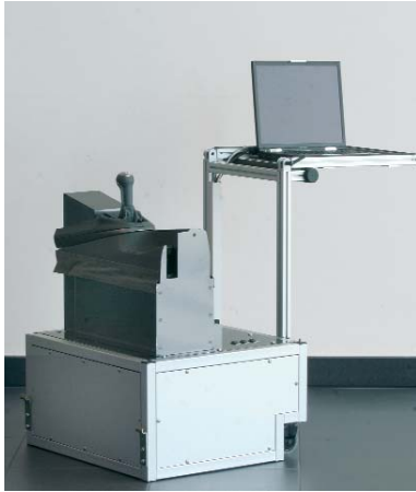
The shifting force simulator: the portable box with manual gearstick, power and control electronics can be used for different types of vehicle.
