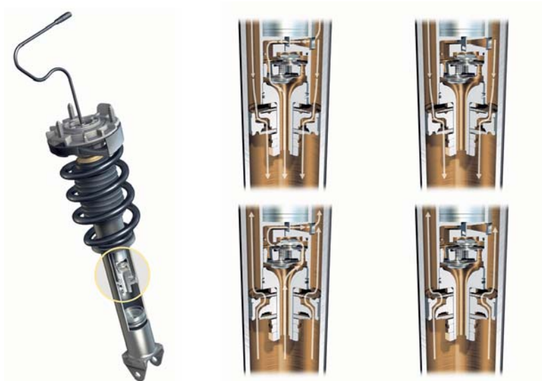
For the first time, the 911 has an active damping system. The PASM consists of map-controlled dampers, a control module and two acceleration sensors.
